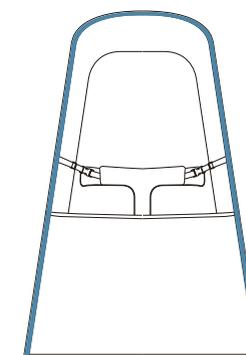
Carefully pass the seat frame through the mesh cover as shown.
